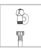
1. Connect the supply pipe by screwing it to a cold water tab using a <sup>3</sup>/<sub>4</sub> gas threaded connection (see *figure*).
